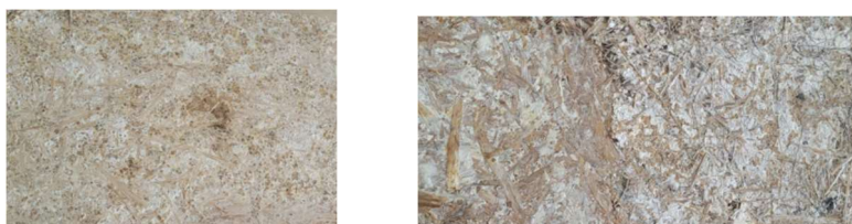
Figure 1. Composite plate made from hemp fibers and mushroom farming waste.
