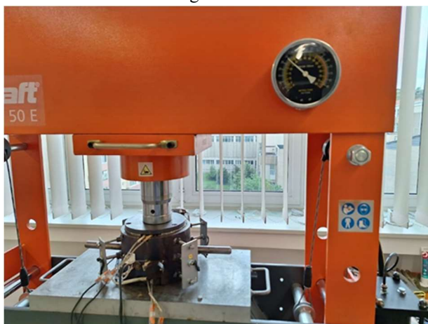
Fig. 2 Composite material plate thermoforming system
